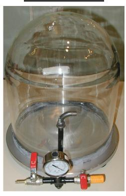
Description: A borosilicate glass domed top bell jar approx 350mm overall height x 300mm ID sits in a Nitrile 'L' seal on to a machined aluminium base plate.
